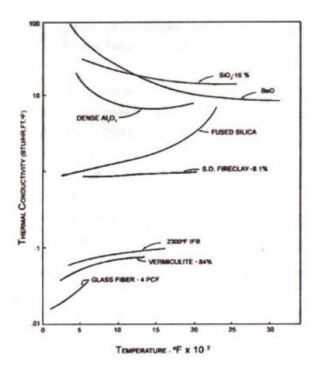
Spinel (MgAl<sub>2</sub>O<sub>4</sub>) for instance, has a thermal conductivity lower than that for either MgO or  $Al_2O_3$ . Another example is reducing the thermal conductivity of a solid by introducing porosity and this is the most common technique of manufacturing insulating refractories
